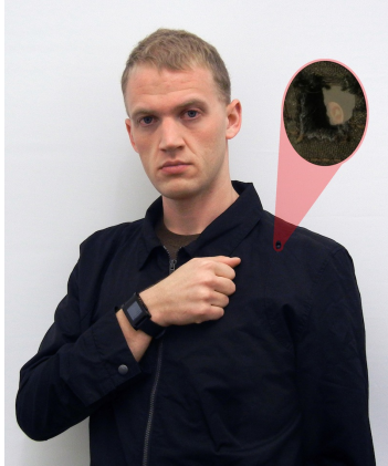
Figure 2: Discreet wearable assistant as a jacket with an internal pocket out from which a camera observes, and a watch, through which private information is communicated to the wearer through glanceable or vibration-encoded text.
